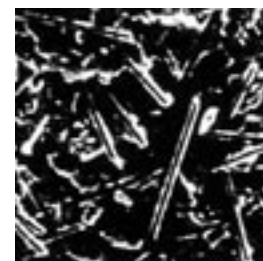
30% glass reinforced nylon 6/6, single gated (24,200 psi)
